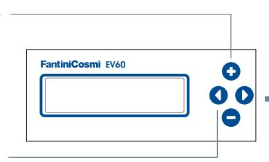
The 2 keys (< and >) are used to enter in the menu and to pass from one page to another.
