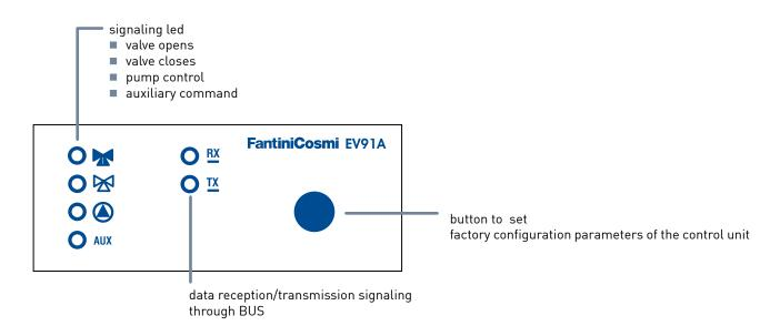
EV91A scope is to obtain a certain AMBIENT TEMPERATURE by measuring the delivery temperature and the external temperature.
